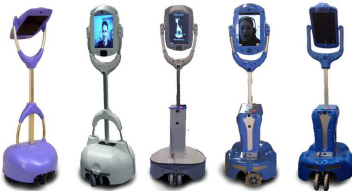
**Figure 1.** Aesthetic evolution of the Giraff over the entire project (from left to right): Giraff 1.0, Giraff 2.0, Giraff 3.0, Giraff 3.2 and Giraff 4.0.
